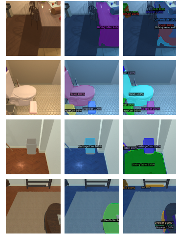
Figure 8: Concept learning visualization. From left to right: the original image, supervised instance segmentation map, and our concept learning results.
